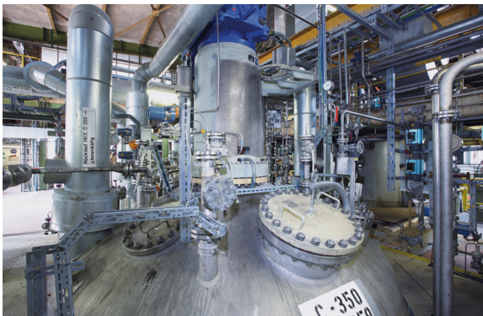
Agitator in a chemical plant
