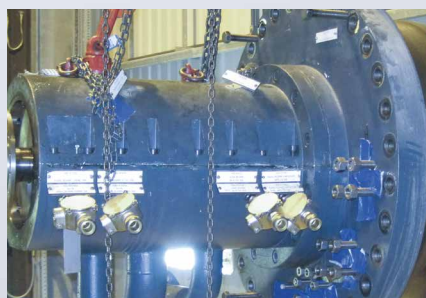
Compressor shaft prior to installation
